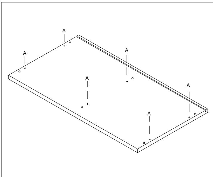
**1.** Place top & bottom inside face up on flat surface. Insert cam bolt A into 5mm holes as shown above.
