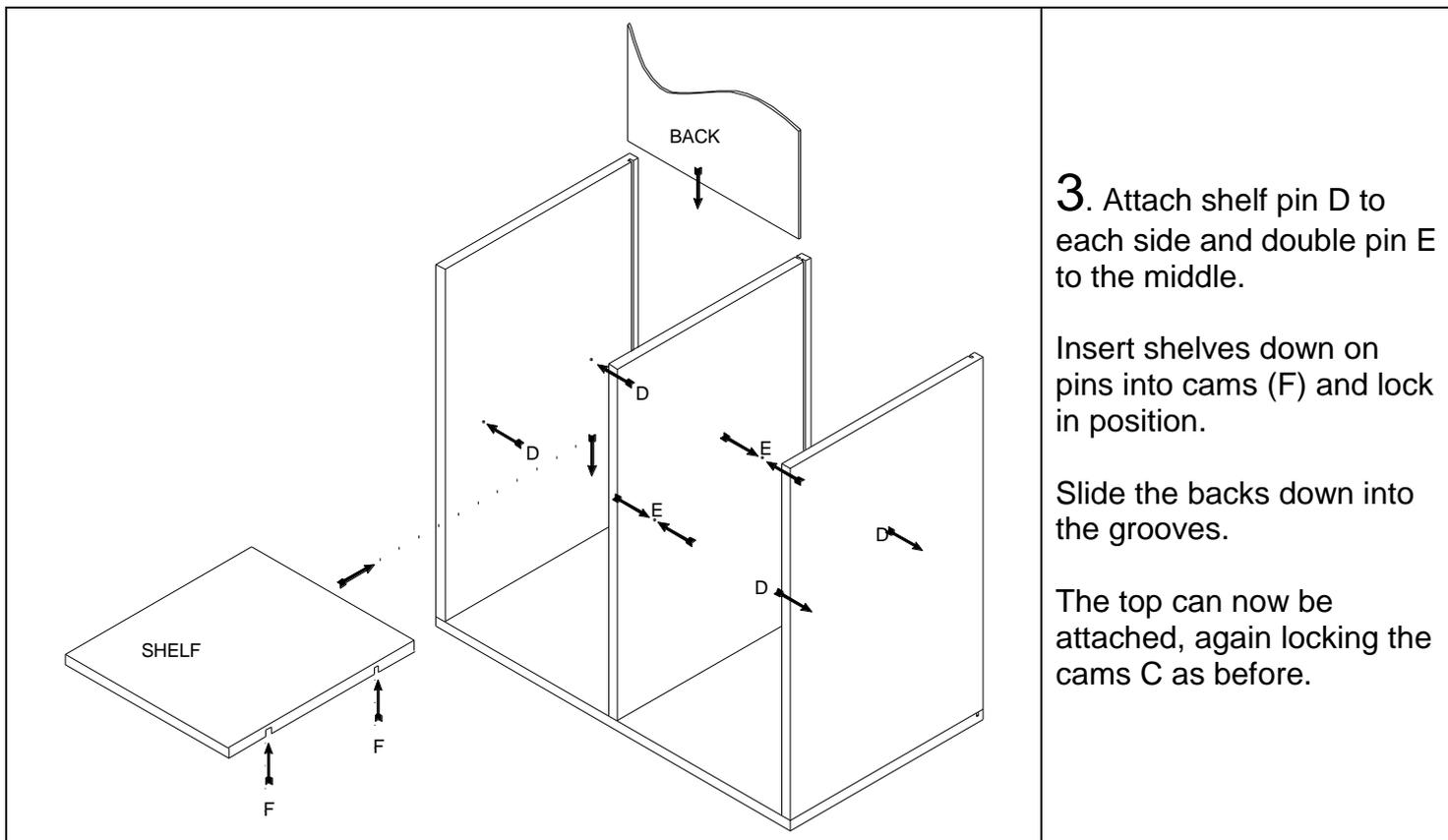
**3.** Attach shelf pin D to each side and double pin E to the middle.
