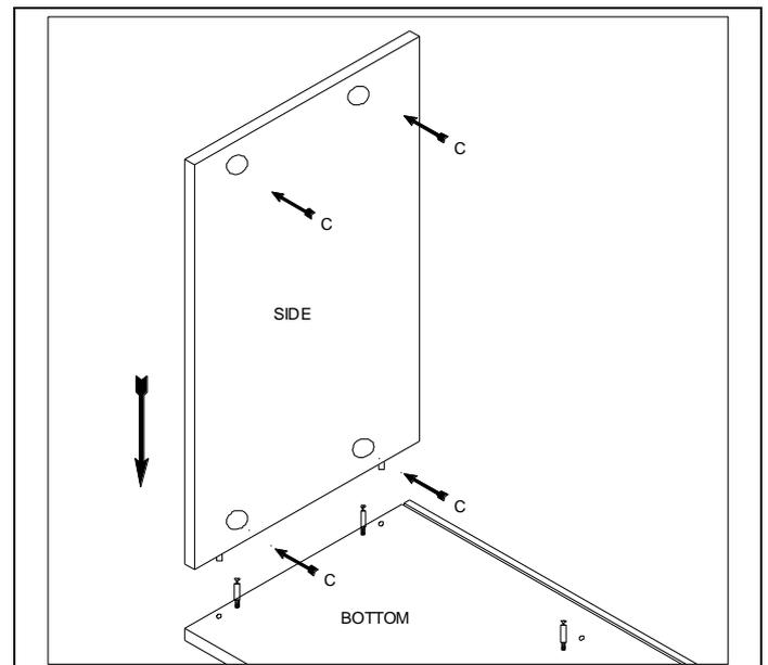
**2.** Insert cam C to 15mm holes on sides and middle. Proceed to assemble from the bottom up turning the cam clockwise to lock.
